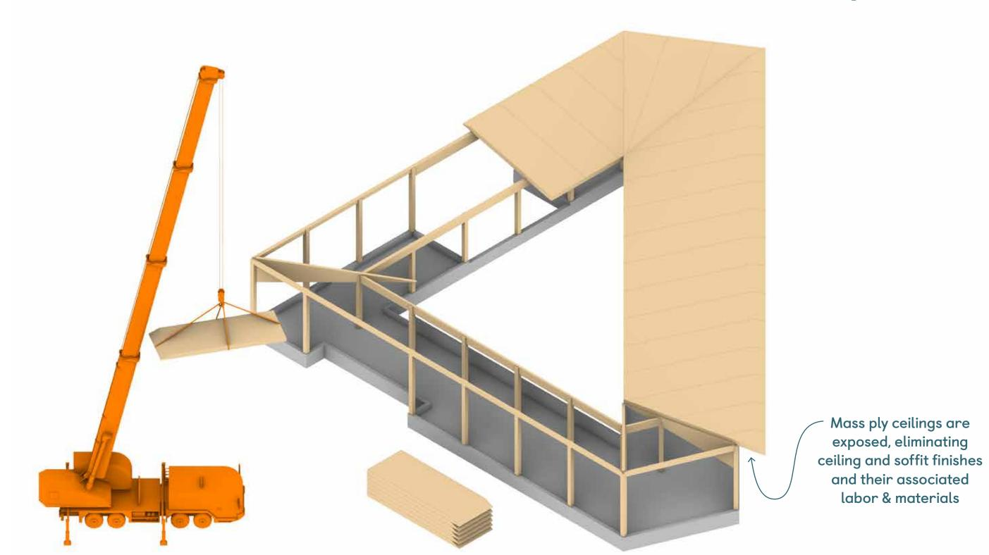
Mass Ply Columns & Beams erect quickly like an assembled kit of parts, minimizing the construction timeline.
